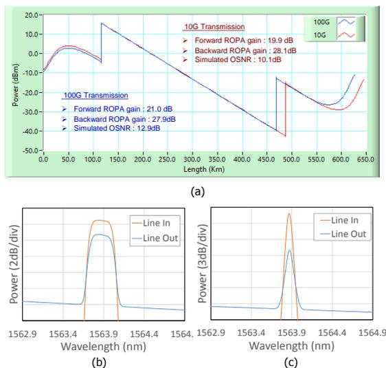
Figure 2. (a) Simulated signal power distribution, Output OSA spectra of (b) 100G, (c) 10G transmission.
