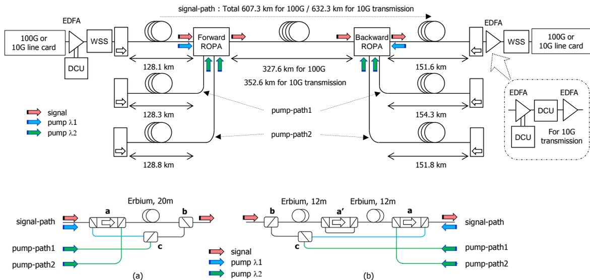
Fig. 1: (TOP) Experimental setup for single 100G/10G channel unrepeated transmission using two additional ROPA pumping fibers. Insert (dashed box) shows the equipment used for 10G transmission. (BOTTOM) Configurations of (a) forward ROPA, (b) backward ROPA. a, a' : hybrid filter (consists of sig/pump Mux, isolator, and sig/pump Mux), b : sig/pump Mux, c : pump  $\lambda_1/\lambda_2$  Mux.
