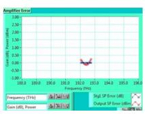
Control loop in action: gain error over 61nm spectrum before and after 135 out of 150 channels are turned off.
