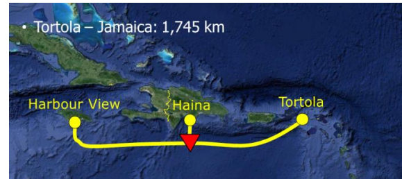
Figure 5: East West Cable redeployment project based on decommissioned Gemini cable.
