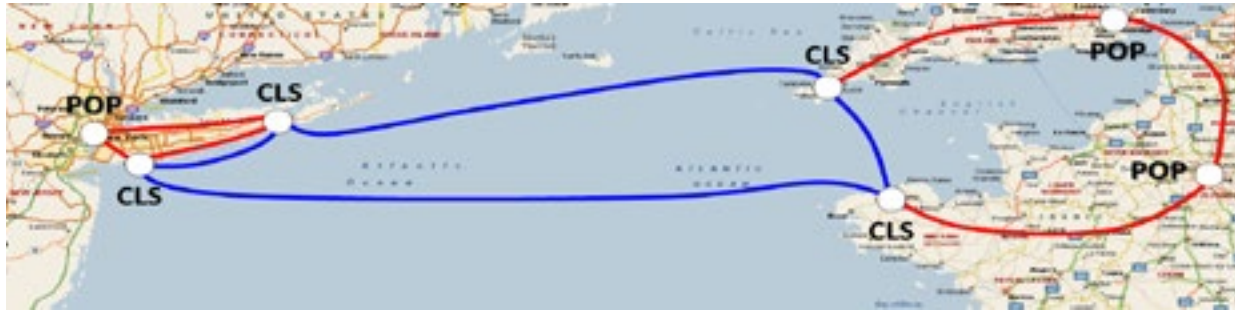
Figure 3: Terrestrial backhaul and subsea networks multiple protection routes for more restoration possibilities.
