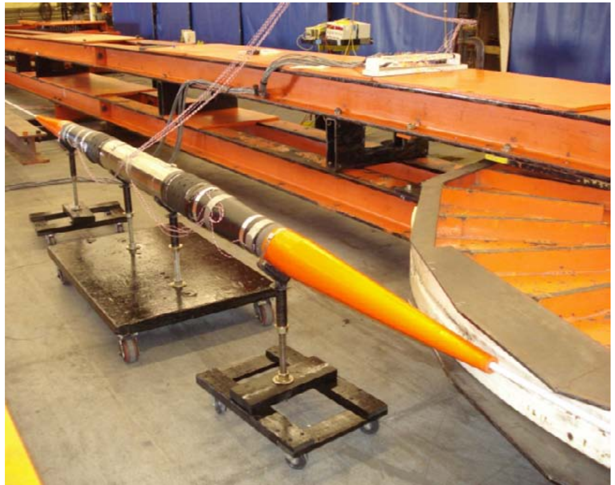
Lightweight repeater undergoing extensive terrestrial test to simulate deployment, handling and recovery
